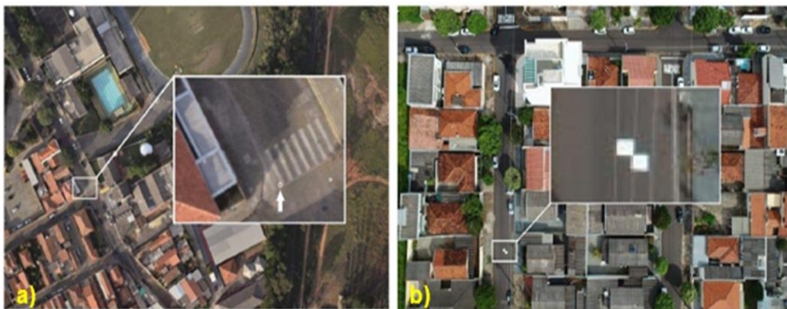
Figura 16: Alvo natural (a) e alvo artificial (b)
