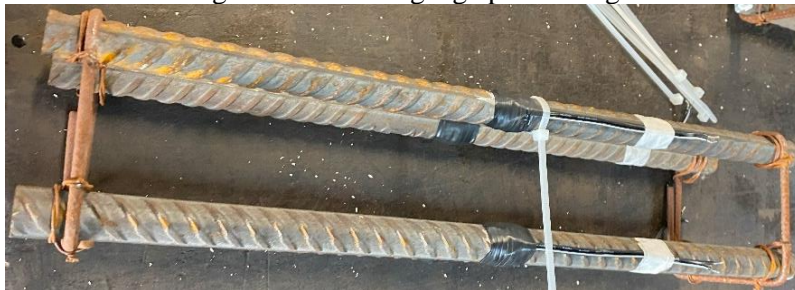
Figure 5.7 - Strain gauge positioning
